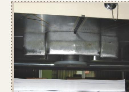
• Magnetic die clamping device enables dies without backing plates to be used.
