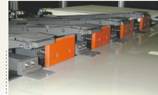
• Paper blank clamping device features air flotation in the lower clamps to allow minor adjustment of the paper stack, which is critical for cut to print operations.
