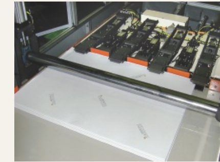
• Roller mechanism ensures material flatness during the cutting process for better position accuracy.
