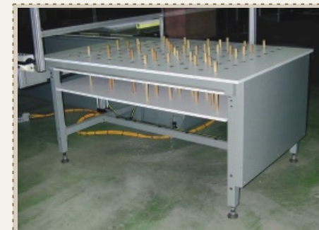
• Cut-part knockout device with a cut-part collecting table.
