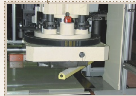
• Die lubrication provides a smooth cut edge and prolongs die life.
